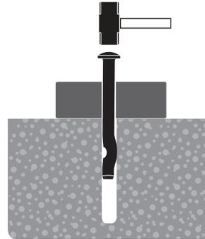
Tap in anchor until seated and flush with surface of fixture.
